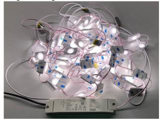
Note that the end of the last string re-attaches to the first string to form a loop. This is to prevent voltage drop to the last string. The driver is now supplying power to both ends.
